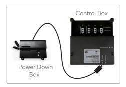
A Sync Cord is included with the base. Not available on Queen, Full or Full-Long size bases. The Sync Cord connects the two control boxes to a single remote for the synchronization of two bases.
